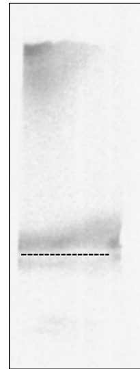
FIG. 7. EUV pinhole image of the discharge at 40 ns before the pinch, recorded at an increased MCP voltage of 6.24 kV. The area of the image corresponds to an area of 1.6 mm wide and 4.2 mm high in the source. The dashed line gives an indication of the position of the surface of the cathode. Like in the visible light images, the real anode position corresponds to the top of the frame, but the region closest to the anode is obstructed from the view. In this image, some EUV emission is visible from the region just outside this obstruction.
